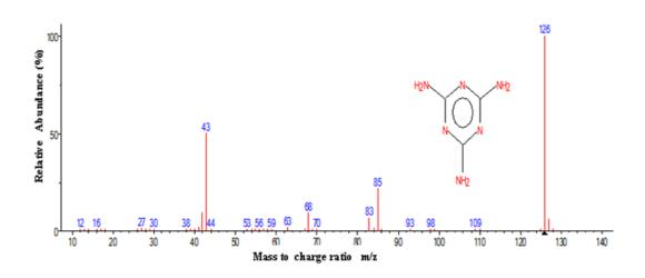
Fig. 6: Mass spectrum of 1,3,5-Triazine-2,4,6-triamine. (RT: 7.85)
