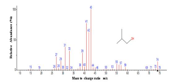
Fig. 7: Mass spectrum of 1-Propanol, 2-methyl. (RT: 9.64)
